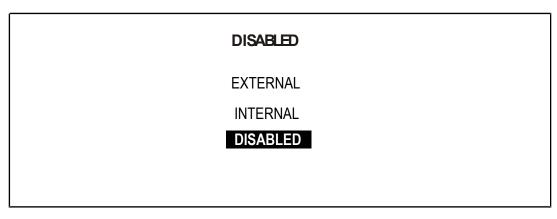
To enable the modem, highlight INTERNAL or EXTERNAL and press SELECT. The Auto Dial screen will return (**Figure 56**) except instead of DISABLED, the message will read INTERNAL or EXTERNAL.
